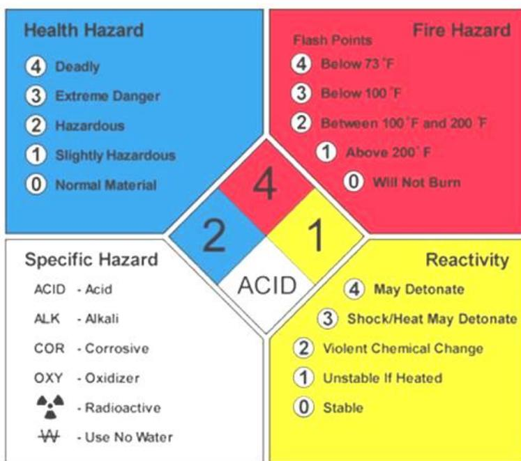
Figure 1: Hazard Diagram
